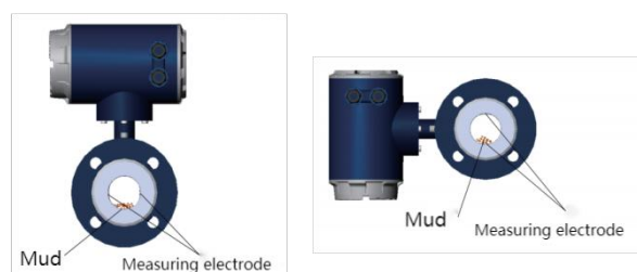
Figure 13 Flowmeter Installation Direction
