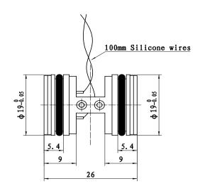
The recommended installation dimension is  $\Phi19^{+0.05}_{+0.02}$  mm
