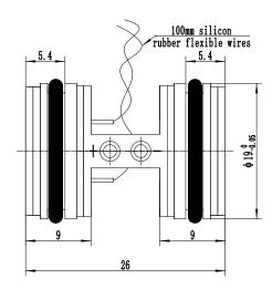
The suggested installation dimension is  $\Phi 19^{+0.05}_{+0.02}$  mm
