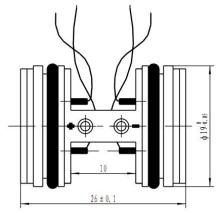
The suggested installation dimension is  $\Phi 19^{+0.05}_{+0.02}\,\text{mm}$
